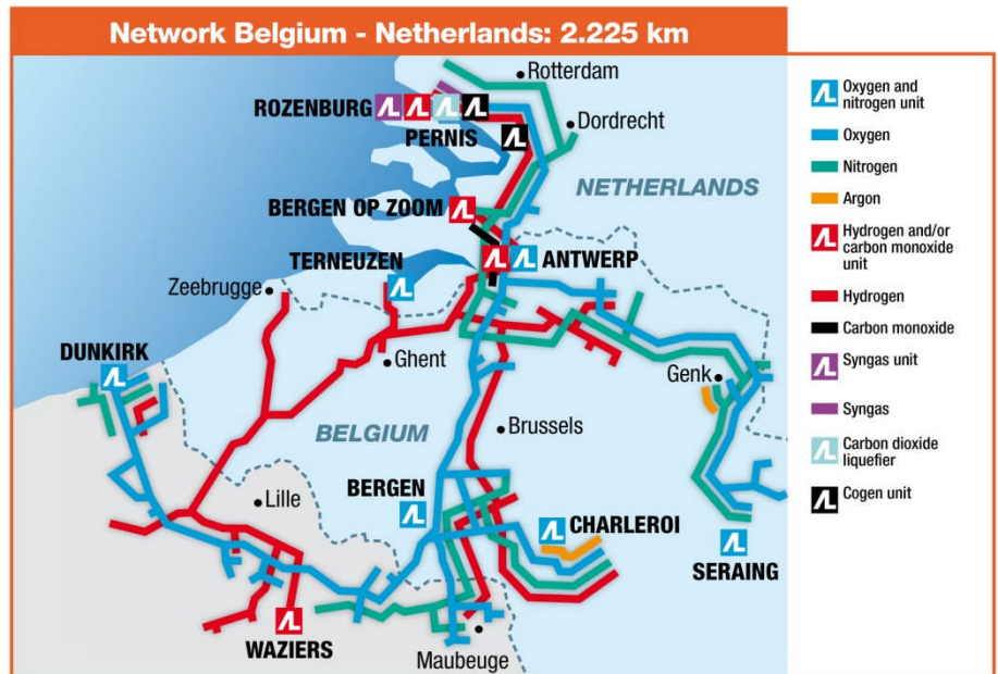
Air Liquide network of pipelines in Benelux
