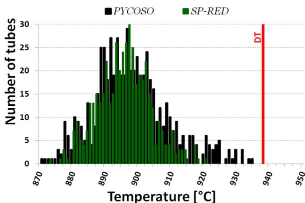
**Figure 5.** Tube temperature distribution in a large scale SMR plant. Comparison between PYCOSO values (in black) before throttling with SP-RED values after throttling 23 burners (in green).
