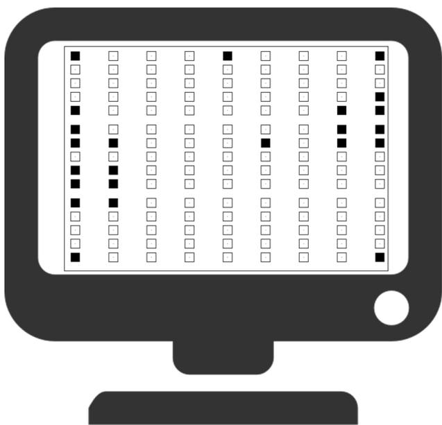
**Figure 4.** Example of throttled burners map with a single throttling condition (throttled burners are represented with full squares and non-throttled burners with empty squares).
