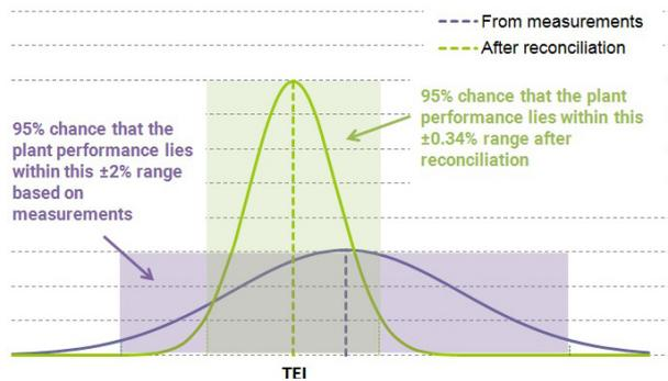
**Figure 1.** Plant thermal efficiency indicator range before and after data reconciliation.
