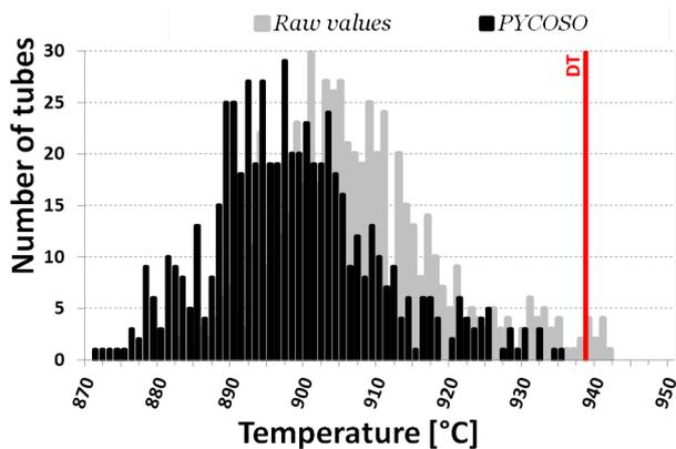
**Figure 3.** Tube temperature distribution in a large scale SMR plant. Comparison between raw values (in grey) and reflected luminance corrected values with PYCOSO (in black).
